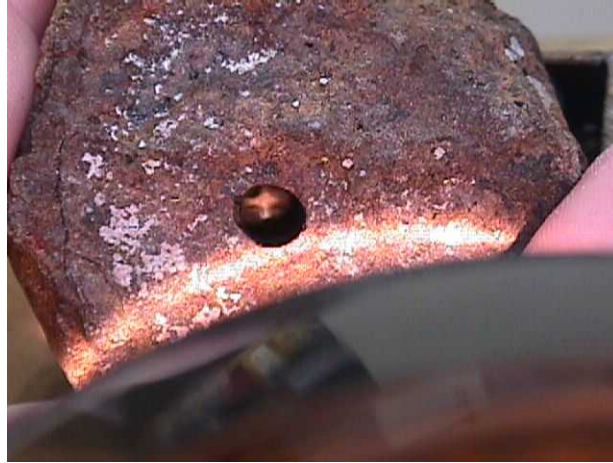
Fig. 8: A basalt stone drilled and coined by microwaves (note the cross-coined in the bottom of the 2-cm deep, 0.5-cm diameter hole)
