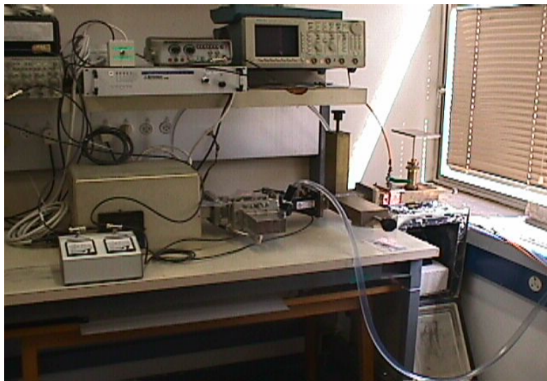
Fig. 2: The experimental microwave-drill apparatus.
