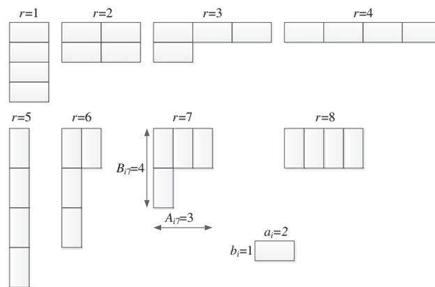
Figure 2. All rectangular configurations for four machines.
