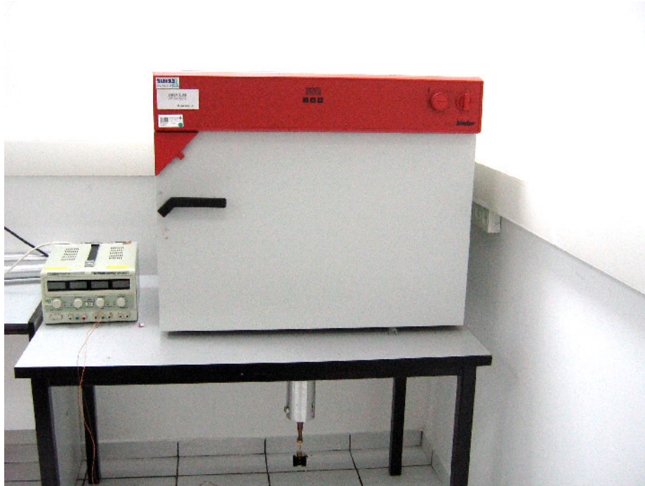
Fig 2: The same Incubator with the radiation source and mode exciter revealed under the table
