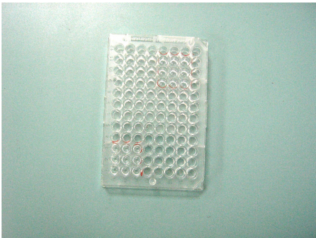
Fig 6: A close up look at the special plastic vessel containing the biological material which is radiation transparent.
