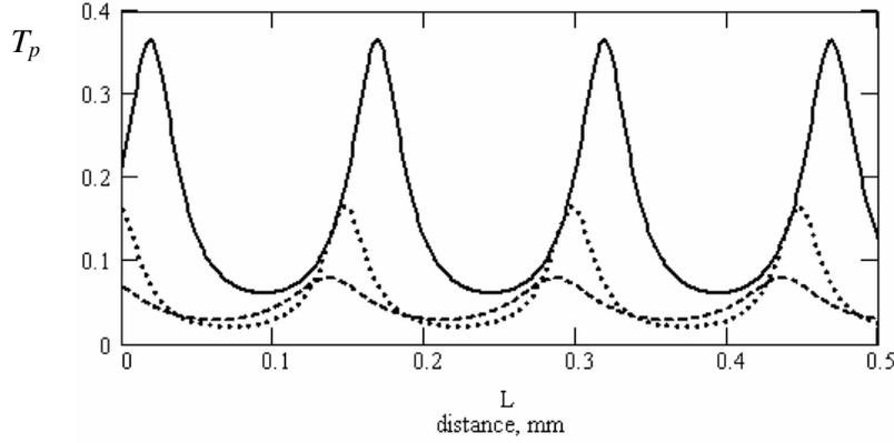
Fig.2 Calculated power transmittance as a function of distance  $L$  between slabs:
