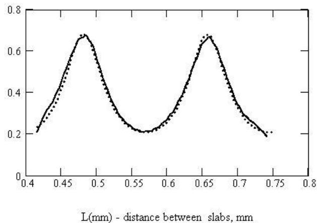
Fig.7 Comparison measured (solid line) and reconstructed transmittances (dotted line) for determined  $\epsilon_r = 9.6$ ,  $\epsilon''_r = 0.04$  ( $\tan\delta = 4.4 \times 10^{-3}$ ) and  $f = 0.855$  GHz.
