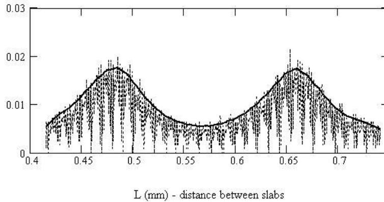
Fig.6 The fragment of smoothing (dotted lone) and the reconstructed envelope (solid line) of the measured data.
