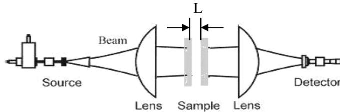
Fig. 3 Schematic of transmitting configuration.
