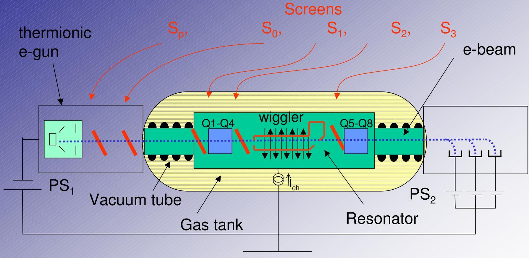
Injector, steering, and focusing coils (1.4 MV)      acceleration      focus and interaction      deceleration      collector
