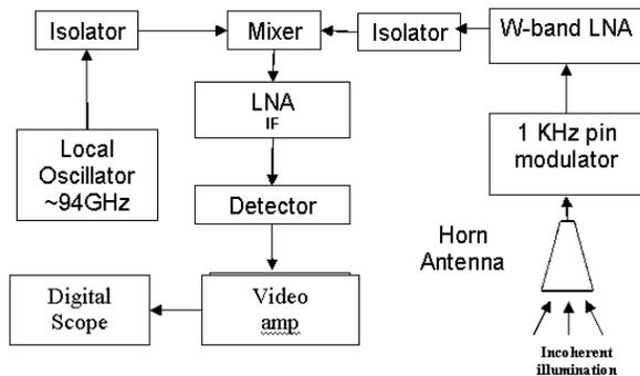
Figure 5: Schematic of the wide band mm-wave sensor.
