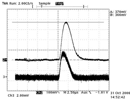
Figure 4: Examples of the detected signals recorded by the digital scope in process of calibration (channel 2 - Rx detector, channel 3 - Tx detector).
