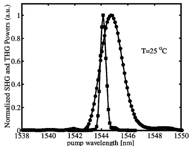
FIG. 2. Normalized SHG (circles) and THG (squares) powers as a function of pump wavelength measured with a GQPS in KTP designed for frequency tripling.
