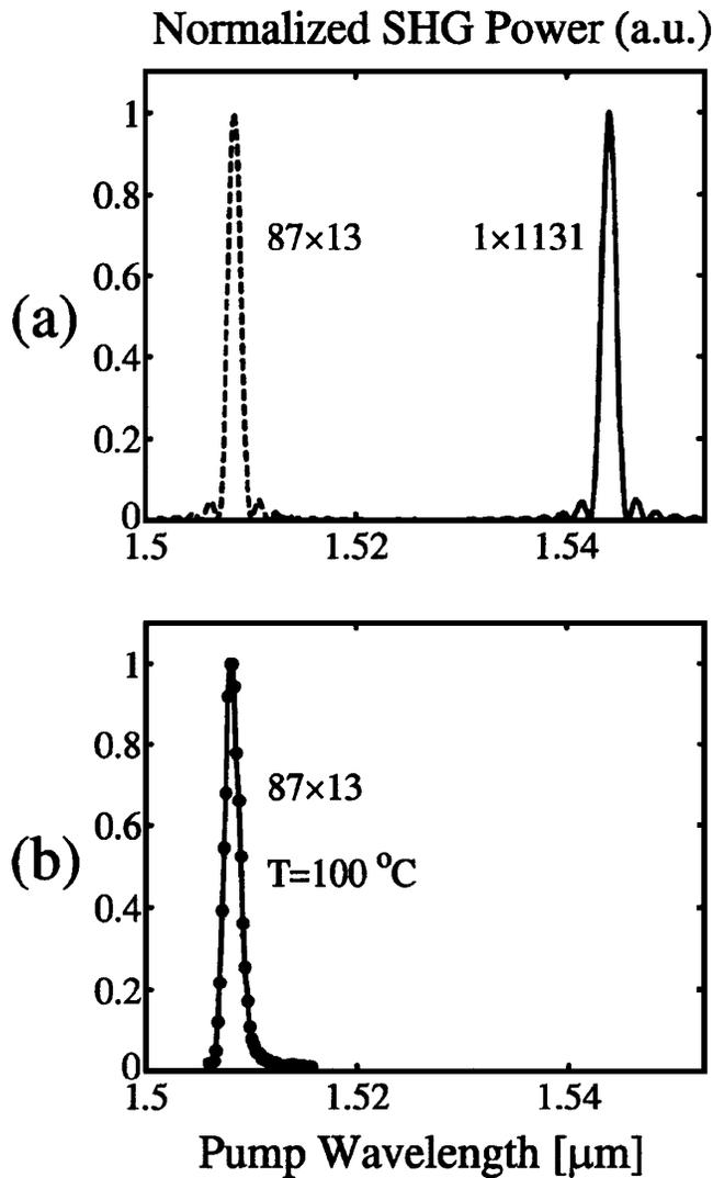
FIG. 3. Normalized SHG power as a function of pump wavelength measured with a GQPS in KTP; (a) calculated without partitioning ( $1 \times 1131$ , solid line) and with partitioning ( $87 \times 13$ , dashed line); (b) measured with partitioning ( $87 \times 13$ ).
