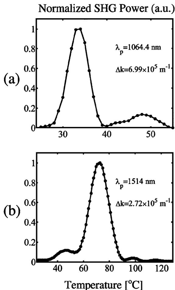
FIG. 1. Normalized SHG powers as a function of crystal temperature measured with a GQPS in KTP designed for dual-wavelength SHG; (a) SHG of 1064.4 nm; (b) SHG of 1514 nm.
