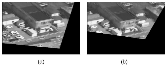
Fig. 2. Accuracy evaluation of plane stabilization. The ground was manually chosen as the reference plane in the first two frames. (a) and (b) display the overlay of frame 1 and frames 20 and 35, respectively, warped toward the first frame. The ground is aligned to a subpixel level, while the roof (above the ground) exhibits parallax effects. The car is duplicated on the road because it was moving while the sequence was taken.
