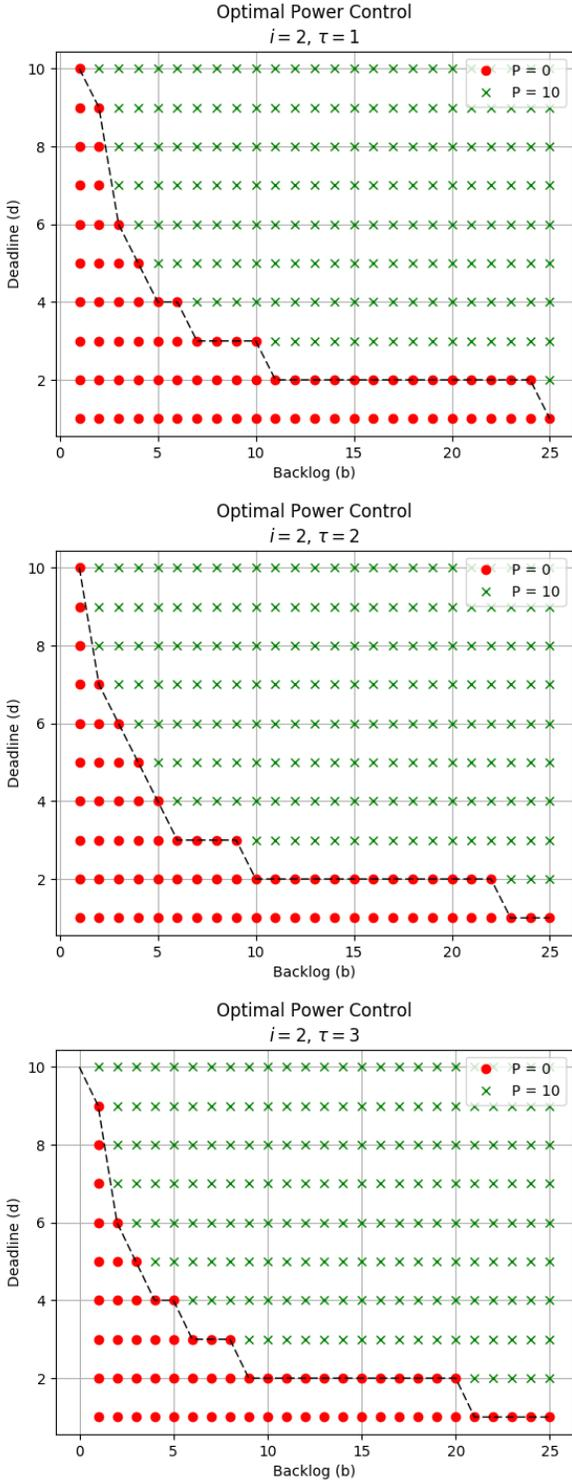
Fig. 4: Optimal power control decision curves for aging interference measurements. Given a fixed channel measurement strategy, it can be shown that the optimal power control remains monotone in  $d$ , as with the more simple models in section III and [13]. Proof omitted here for space, but similar to that of [13].
