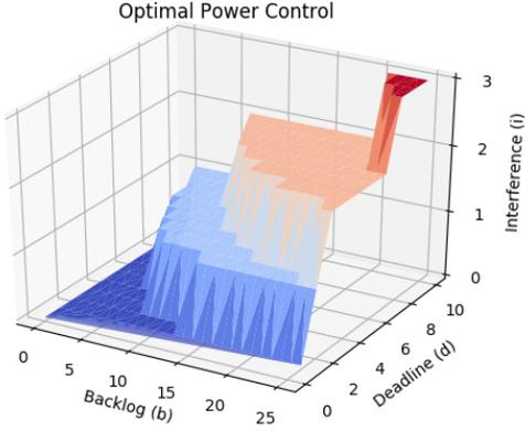
Fig. 3: Binary power control decision surface. States above the control surface represent a low power or transmitter idle decision, and states below represent a high power or active transmission decision.
