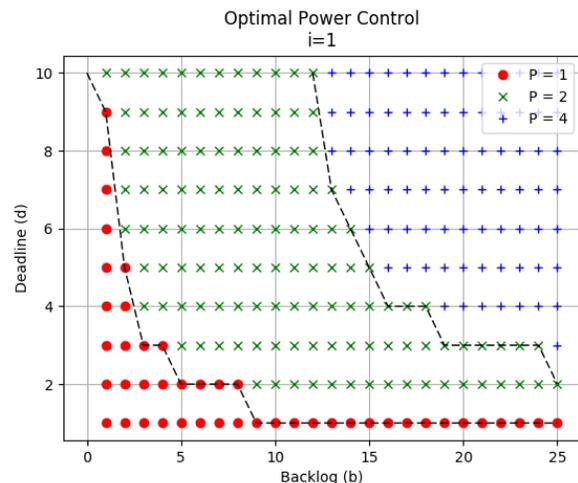
Fig. 2: Ternary power control decision curves. Interference is measured in every time step, and a wider range of allowable transmission powers is considered.
