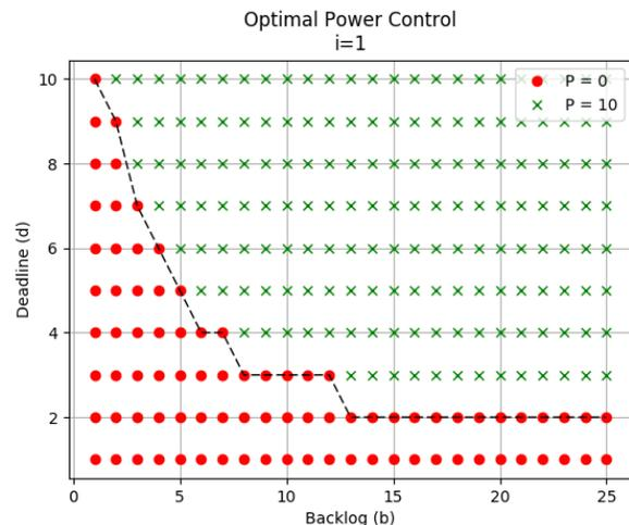
Fig. 1: Binary power control decision curve for a fixed interference level. The interference level is sensed in every time step, and the optimal power control is derived subject to the known interference.
