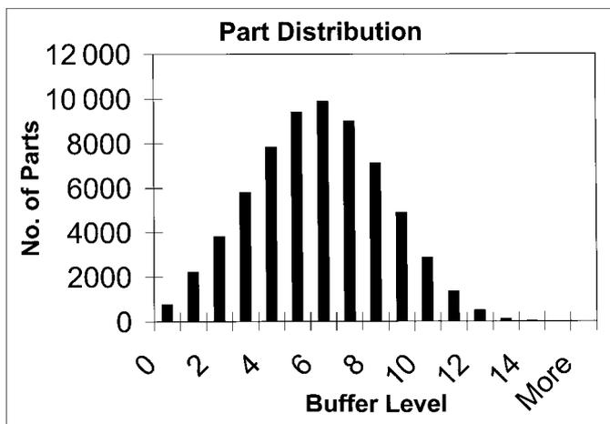
**Fig. 4.** Distribution of parts in the first buffer at steady-state.
