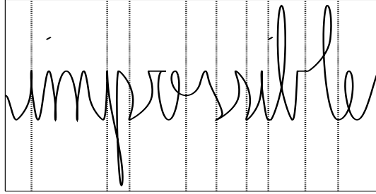
Figure 4: Temporal segmentation of the word impossible . The segmentation is performed by evaluating the probabilities of the APFAs which correspond to the letter constituents of the word.
