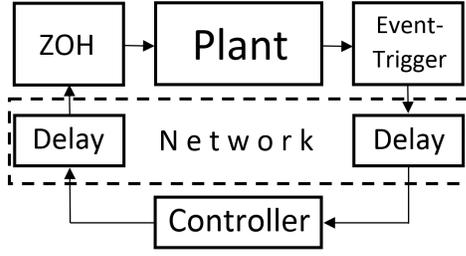
Fig. 1. A system with network-induced delays
