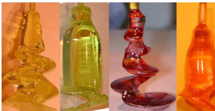
**Fig. 1** From left to right: DyScO<sub>3</sub> crystal showing an extreme case of spiral growth, DyScO<sub>3</sub> crystal with later onset of spiral growth, SmScO<sub>3</sub> with very distinctive spiral growth, SmScO<sub>3</sub> crystal with later onset of spiral growth. (Online color at [www.crt-journal.org](http://www.crt-journal.org))
