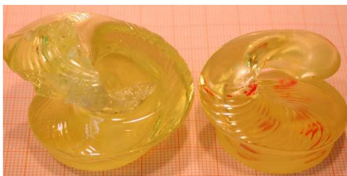
**Fig. 2** DyScO<sub>3</sub> crystals grown in opposite rotation directions. The formed spirals show opposite turns. (Online color at [www.crt-journal.org](http://www.crt-journal.org))
