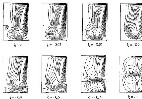
FIG. 1. Counter-rotating bottom. Streamlines. Here  $Re=1500$ ,  $\gamma=1.5$ ,  $0\geq\xi\geq-1$ .
