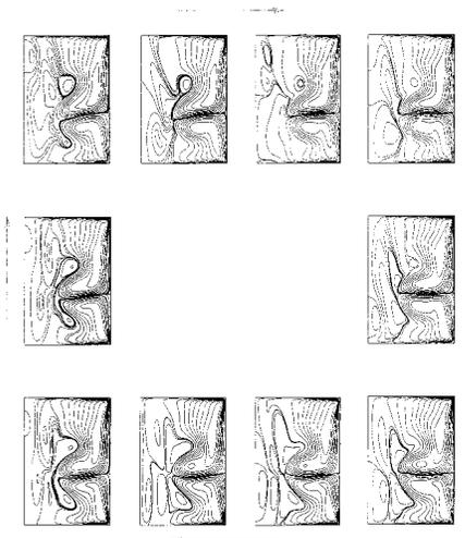
FIG. 17. Instantaneous streamlines of the meridional flow plotted for equal time intervals  $0.1T$  covering the complete period  $T=15.25$ .  $\gamma=1.5$ ,  $\xi=0.8$ , and  $Re=4200$ . Calculation with the finite volume method using a  $150 \times 150$  stretched grid.
