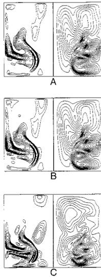
FIG. 16. Changes in the patterns of the perturbations of  $u_\varphi$  (the left part of each plot) and of  $\psi$  (the right part of each plot) at  $\xi=0.54$  corresponding to three values of  $Re_{cr}$ . (a)  $Re_{cr}=3463$ ; (b)  $Re_{cr}=4326$ ; (c)  $Re_{cr}=4632$ .
