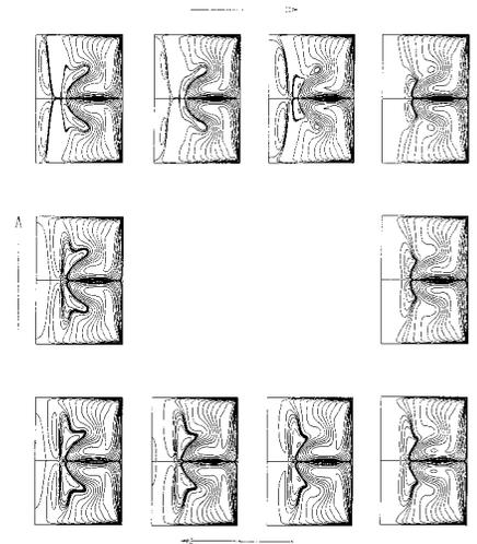
FIG. 18. Instantaneous streamlines of the meridional flow plotted for equal time intervals  $0.1T$  covering the complete period  $T=13.01$ .  $\gamma=1.5$ ,  $\xi=1$ , and  $Re=3845$ . Calculation with the finite volume method using a  $150 \times 150$  stretched grid.
