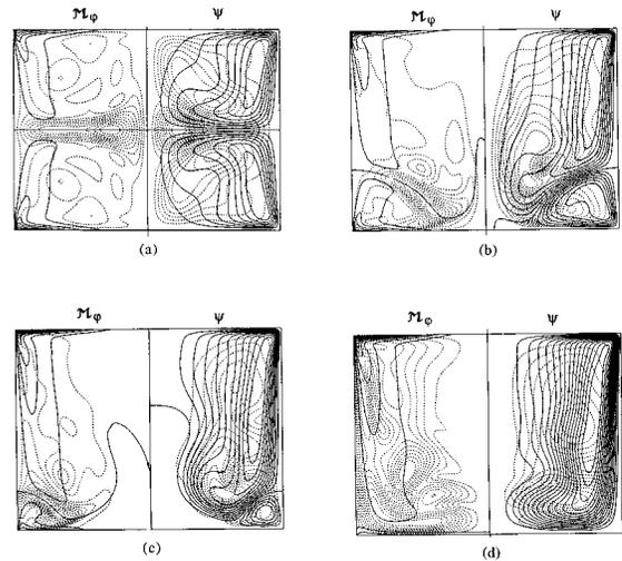
FIG. 11. Isolines of the rotational moment  $\mathcal{M}_\varphi$  (the left part of each plot) and the streamfunction  $\psi$  (the right part of each plot) at the critical point (solid lines) and isolines of the corresponding perturbations (dashed lines). Counter-rotation,  $\gamma=1.5$ . (a)  $\xi = -1$ ,  $Re_{cr} = 1646$ ; (b)  $\xi = -0.64$ ,  $Re_{cr} = 2905$ ; (c)  $\xi = -0.49$ ,  $Re_{cr} = 3158$ ; (d)  $\xi = -0.05$ ,  $Re_{cr} = 2585$ .
