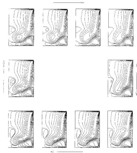
FIG. 12. Instantaneous streamlines of the meridional flow plotted for equal time intervals  $0.1 T$  covering the complete period  $T=19.21$ .  $\gamma=1.5$ ,  $\xi=-0.6$ , and  $Re=3200$ . Calculation with the finite volume method using a  $75 \times 75$  stretched grid.
