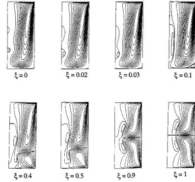
FIG. 9. Streamlines of meridional flow for  $Re=2000$ ,  $\gamma=2.5$ ,  $0 \leq \xi \leq 1$ .
