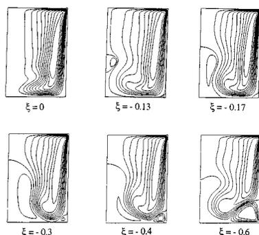
FIG. 4. Counter-rotating bottom. Streamlines. Here  $Re=3800$ ,  $\gamma=1.5$ ,  $0 \geq \xi \geq -0.6$ .
