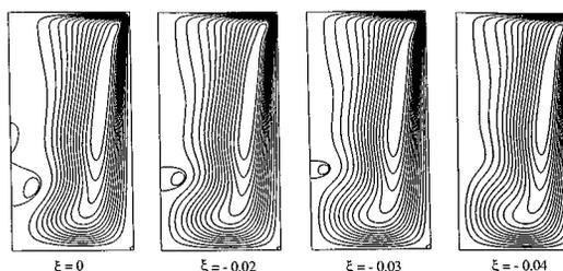
FIG. 2. Counter-rotating bottom. Streamlines. Here  $Re=2000$ ,  $\gamma=2.0$ ,  $0\geq\xi\geq-0.04$ .
