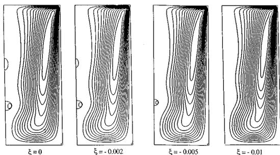
FIG. 3. Counter-rotating bottom. Streamlines. Here  $Re=2000$ ,  $\gamma=2.5$ ,  $0 \geq \xi \geq -0.01$ .
