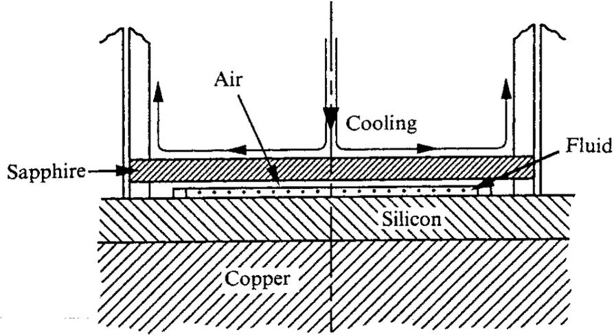
Figure 1: Sketch of the experimental set-up (from [1]); the liquid is situated on the (heated) silicon block and separated from the (cooled) sapphire block by a small air gap.
