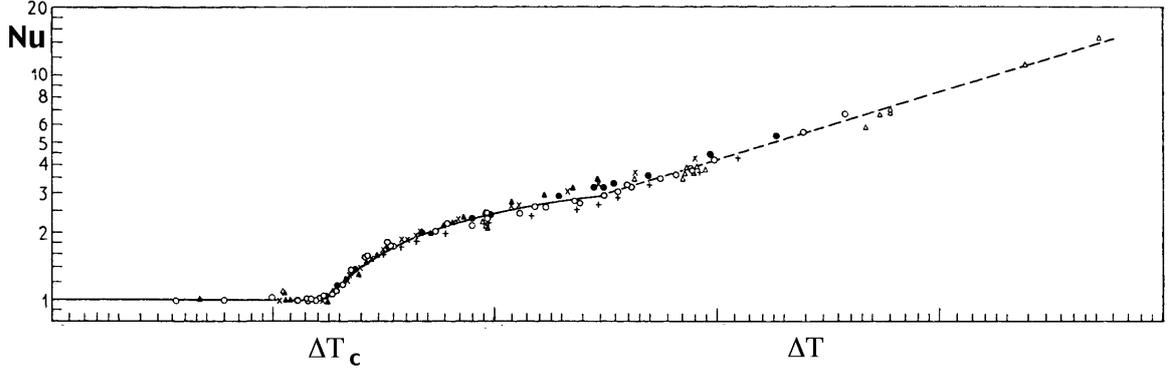
Figure 2: Plot of the Nusselt number (see text) as a function of the vertical temperature gradient  $\Delta T$  (from [2]);  $Nu = 1$  if the heat transport is by conduction only and  $Nu$  increases if there is convection in the liquid;  $\Delta T_c$  is the critical temperature gradient.
