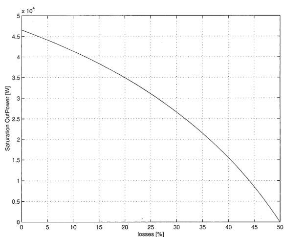
Fig. 5. The FEL output power  $P_{out}$  as a function of the out-coupling parameter of the resonator  $T_m$ , for different internal loss values  $L$ .
