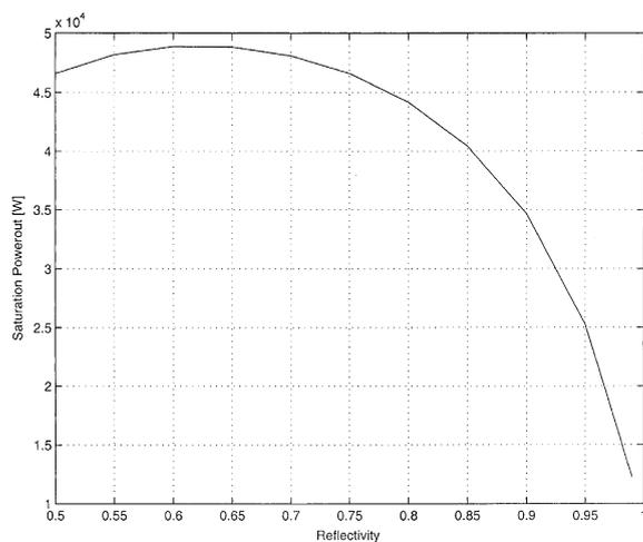
Fig. 4. The total power extracted from the e-beam  $\Delta P$  and the power at the end of the resonator  $P(L_w)$  as a function of the resonator reflectivity  $R$ .
