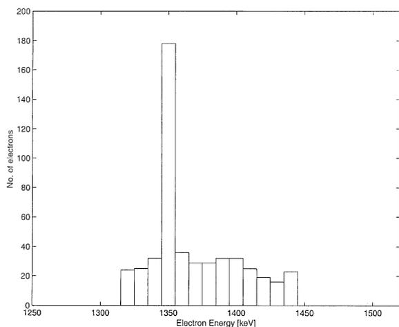
Fig. 3. Electron energy distribution at minimal electron energy spread conditions ( $R = 50\%$ ).
