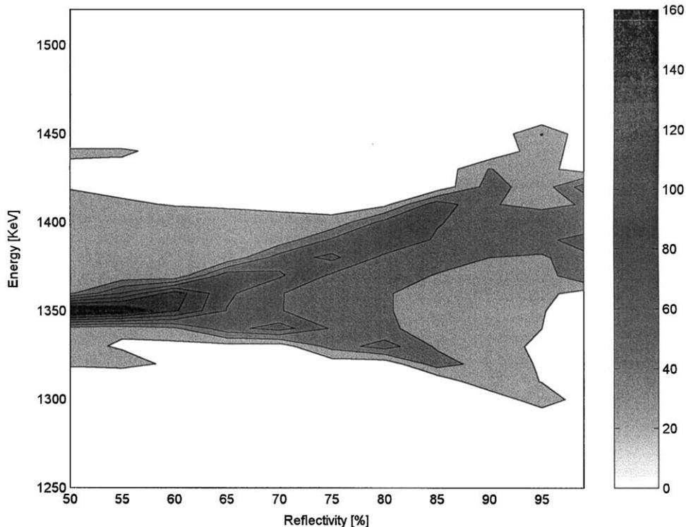
Fig. 2. Electron beam energy spread as function of the resonator reflectivity  $R$  (the gray scale indicates the number of electrons per energy interval).
