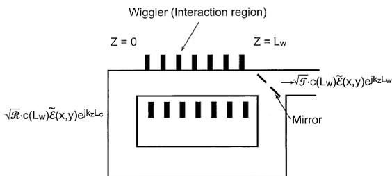
Fig. 1. A schematic of an FEL oscillator.
