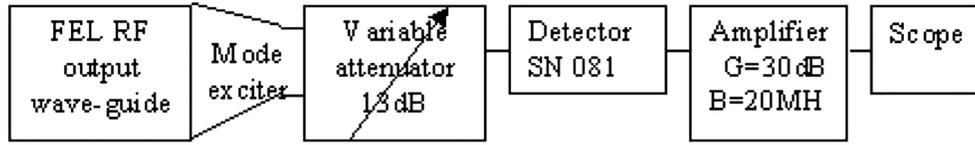
FIG. 2. Measurement setup.
