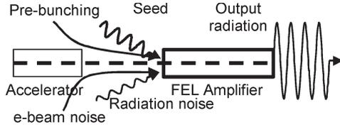
Fig. 4. Coherent and incoherent radiations and beam modulation input signals at the FEL amplifier input. The amplified signal output power is partially coherent.
