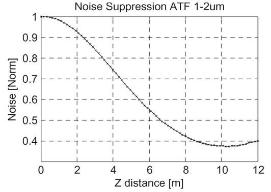
Fig. 2. ATF simulation results: Current noise reduction for 1–2  $\mu\text{m}$  for a Gaussian beam.
