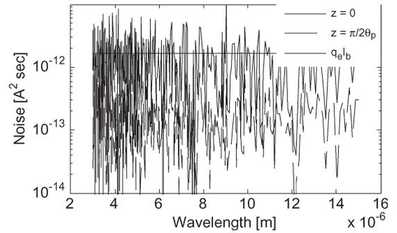
Fig. 3. Noise as a function of wavelength in a logarithmic scale according to the ATF beam parameters. The constant line represents the classical current shot noise for comparison.
