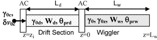
Fig. 1. FEL system composed of a free drift e-beam section, (AC) acceleration sections, and a wiggler section.
