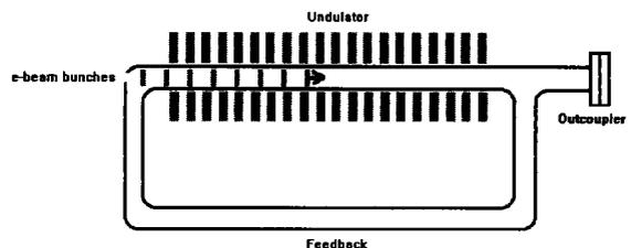
Fig. 1. Schematic illustration of a super-radiant free-electron laser oscillator.
