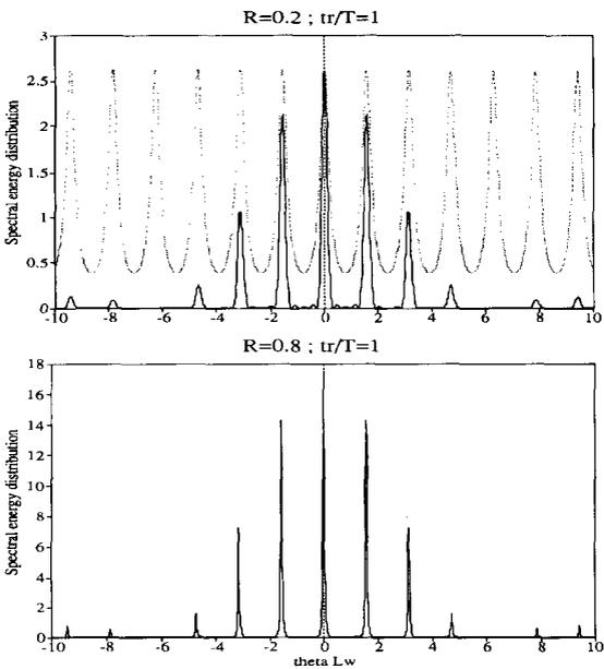
Fig. 4. The line-shape of the out-coupled radiation when a super-radiant emission (of  $N = 5$  bunches, duty-cycle  $\tau_{\text{sp}}/T = 25\%$ ) is circulating in a resonator ( $t_r = T$ ). (a) Finesse  $F = 1.8$  smaller than the number of bunches  $N = 5$ . (b) Finesse  $F = 14$  higher than the number of bunches  $N = 5$ .
