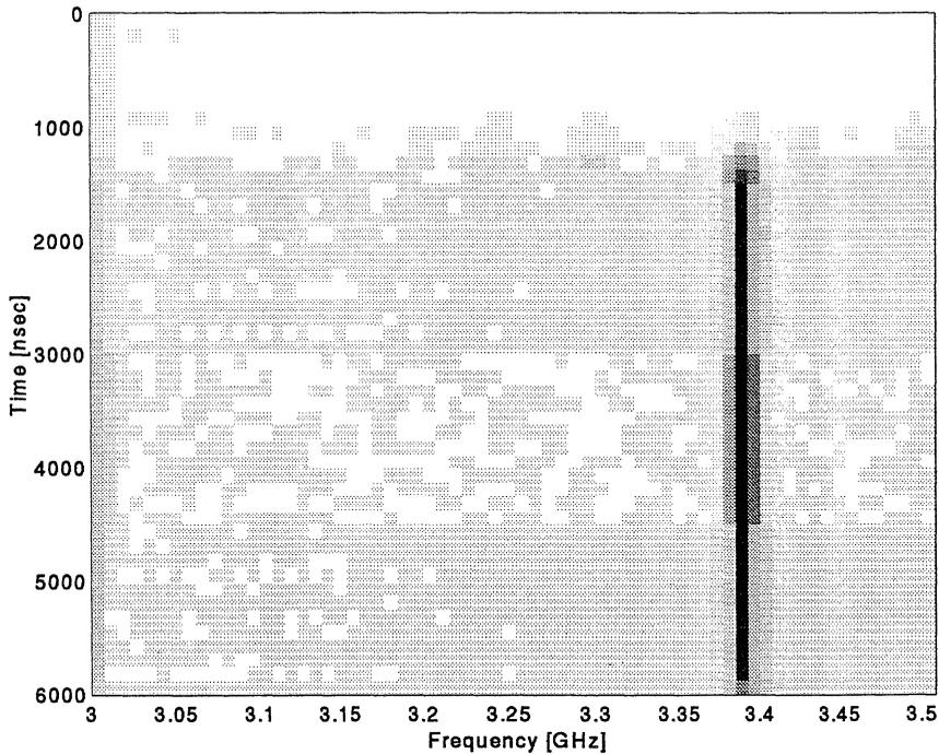
Fig. 5. Time evolution of the FEM radiation near waveguide cutoff frequency.
