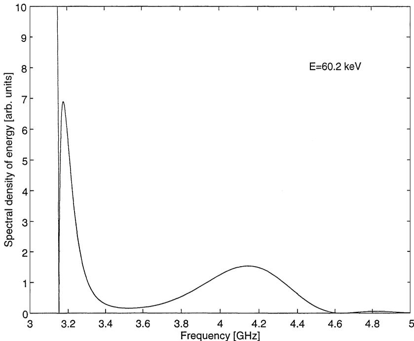
Fig. 3. Spectral density of radiated energy (in arbitrary units) versus frequency.
