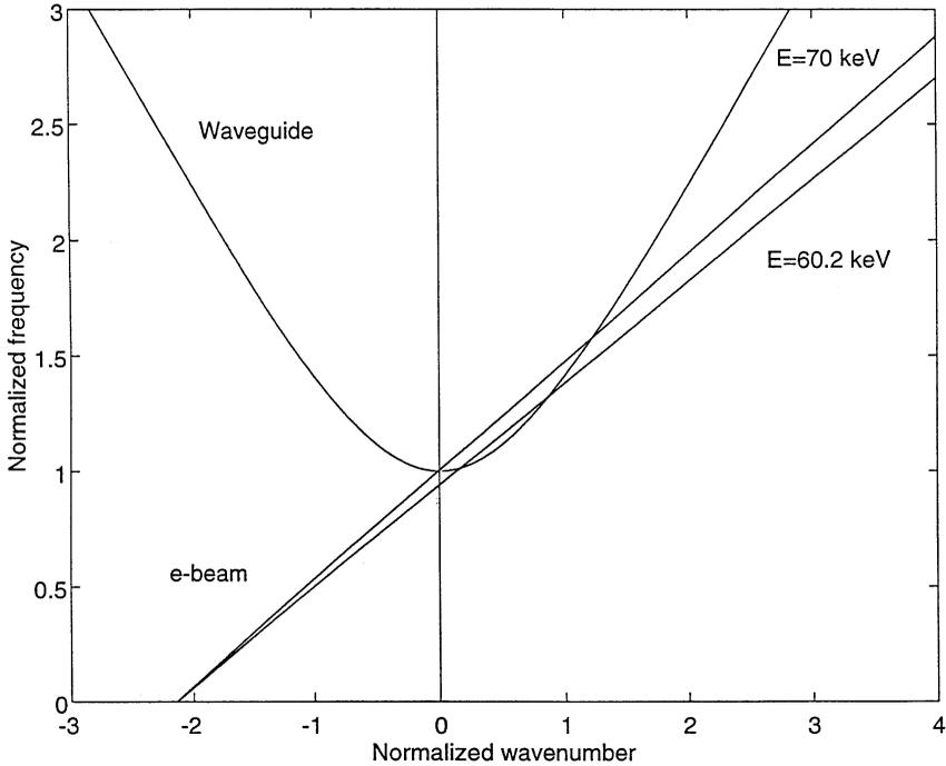
Fig. 1. Normalized frequency  $\bar{\omega} = \omega/\omega_c$  as a function of normalized wave number  $\bar{k}; \bar{k} = k_{10}/(\omega_c/c)$  for the waveguide TE<sub>10</sub> mode, and  $\bar{k} = (\omega/V_z - k_w)/(\omega_c/c)$  for the e-beam mode.
