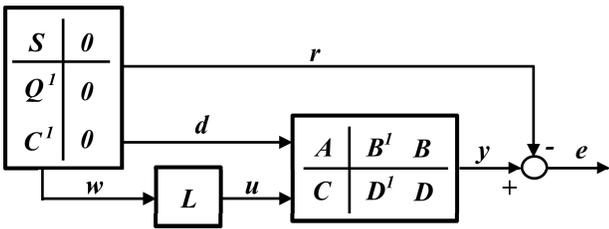
Figure 1. The closed-loop system corresponding to the state feedback regulator problem. The closed-loop system is not asymptotically stable, but the error is in  $L_\alpha^2([0, \infty); Y)$  with  $\alpha < 0$ , like the output of an exponentially stable system.
