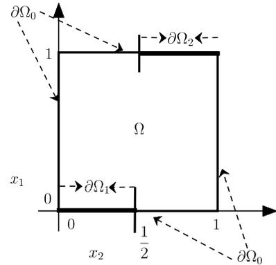
Figure 4. The rectangular domain  $\Omega$ . The part of the boundary  $\partial\Omega_0$  is insulated. The control signal is applied on the rest of the boundary.
