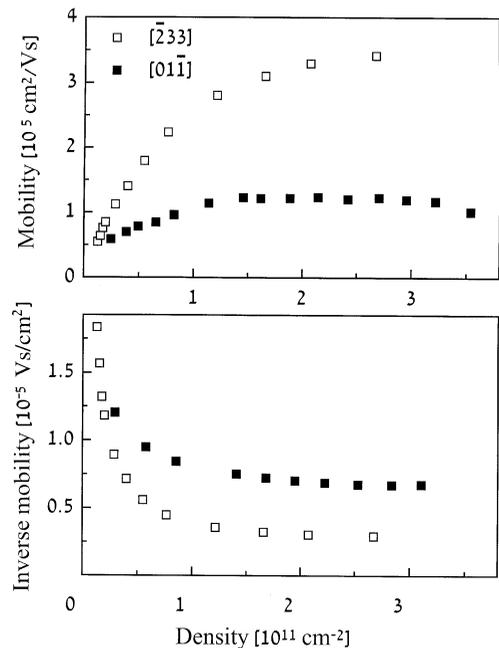
Fig. 3. The mobilities,  $\mu_1$  and  $\mu_2$  measured in Hall bars in the  $[0 1 \bar{1}]$  and  $[\bar{2} 3 3]$ , directions of the (3 1 1)A plane, respectively. In the upper panel,  $\mu_1$  and  $\mu_2$  versus density. In the lower panel, the respective inverse quantities are plotted.
