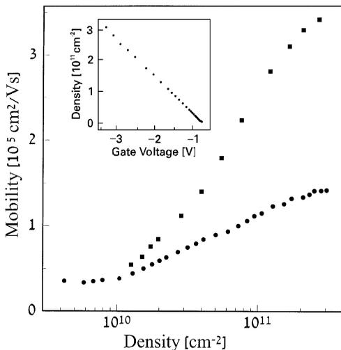
Fig. 2. Mobility of the 2DHG in a p-ISIS, plotted versus its density  $p$ . Data are shown for 6.2 (circles) and 1.6 K (squares). The inset shows, the variation of Hall density with  $V_b$ .
