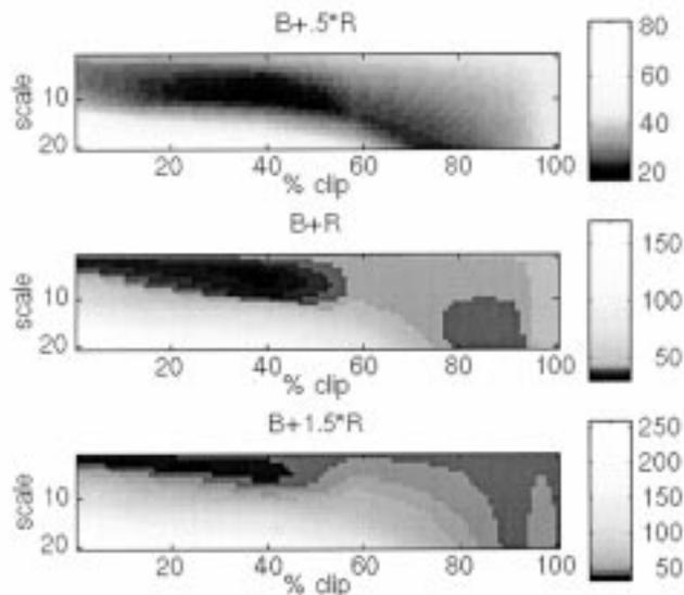
Fig. 5. Error surfaces for three different weighting constants. Black regions indicate low error with an increase in error at the brighter regions.
