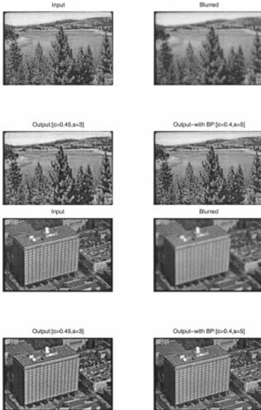
Fig. 9. Enhancement results on two natural scenery, gray level images. In each case, top left image is the original, high-resolution image (“ideal”), top right is the input blurred image, bottom left is the enhanced result using the first parameter set, and bottom right is the enhanced result using the second parameter set.
