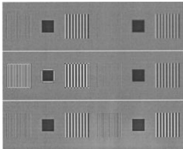
Fig. 15. Global enhancement versus local enhancement. The original input and a blurred version are presented top row, left and right, respectively. Results of the global enhancement scheme are presented in the center row. The results of adaptive enhancement are shown on the bottom.
