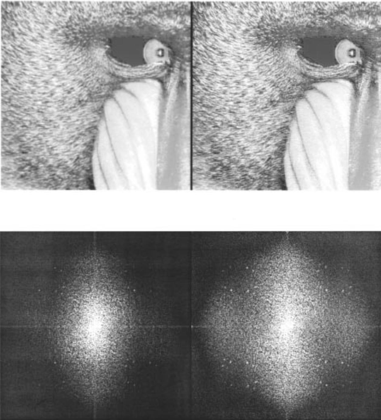
Fig. 10. Given and enhanced images, left to right, respectively, together with their corresponding power spectrum characteristics (bottom). It is evident that the input power spectra is augmented. The enhancement process actually extrapolates to higher frequencies, thus producing the satisfying enhanced result.
