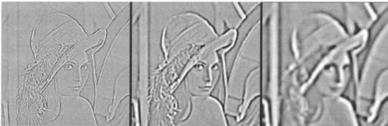
Fig. 1. Multiscale sequence of edge maps. Presented from left to right are the Laplacian pyramid components:  $L_0$ ,  $L_1$ , and  $L_2$ , respectively.
