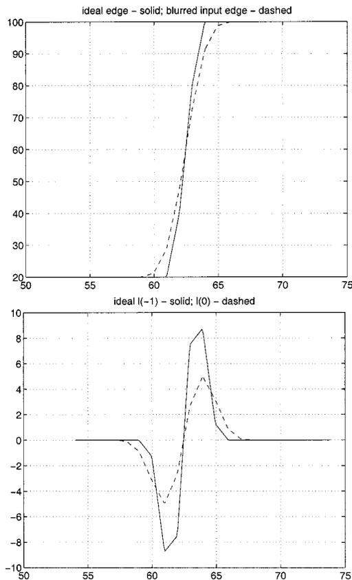
Fig. 7. Top: Input curves, ideal step edge (solid) and input blurred edge (dashed). Bottom: Corresponding Laplacians, ideal  $L_{-1}$  (solid), and extracted  $L_0$  (dashed).
