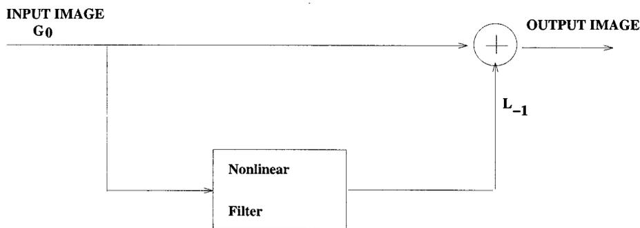
Fig. 2. Basic diagram of the image enhancement algorithm.
