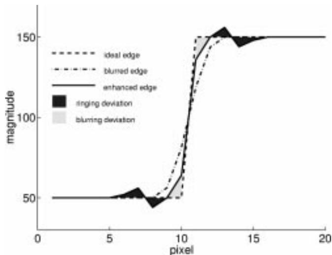
Fig. 4. Blurring and ringing deviations for an ideal edge blurred by a 5-tap Gaussian filter.
