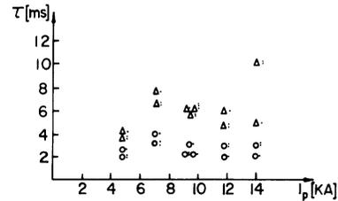
Fig. 7. Time  $\tau$  from arc initiation to beginning of first arc column motion (○) and to the motion of last stationary arc column (Δ), plotted as function of  $I_p$ , peak arc current.
