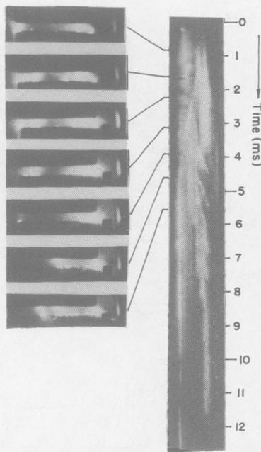
Fig. 4. Streak and frame photography of the arc with external magnetic field. Peak values for current and magnetic field are 9.3 kA and 0.06 T, at 2.9 ms, respectively. Initial capacitor voltage 200 V.
