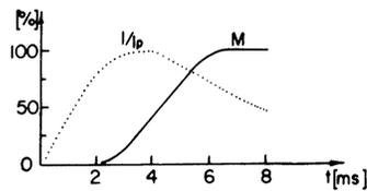
Fig. 8. The ratio  $M$  between the number of moving columns and total number of arc columns, and  $I/I_p$ , the ratio between the momentary current and peak current, as function of time.
