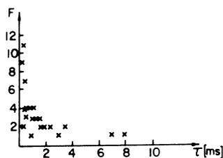
Fig. 10. The number of cyclic repetitions of arc columns  $F$  as function of  $\tau$ , the duration of a single arc column movement.
