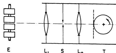
Fig. 3. Schematic drawing of streak camera.
