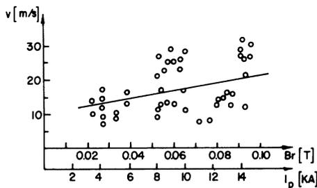
Fig. 9. The velocity of arc columns as function of peak current  $I_p$ , or peak magnetic field  $B_r$ .
