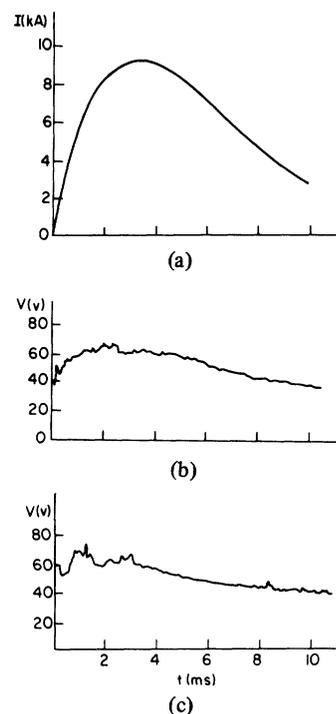
Fig. 2. Current  $I$ , and voltage  $V$ , waveforms as a function of time  $t$ , for 200-V initial capacitor voltage. (a) Current. (b) Arc voltage, with external magnetic field of  $6.5 \times 10^{-6}$  T/A. (c) Arc voltage without external magnetic field.
