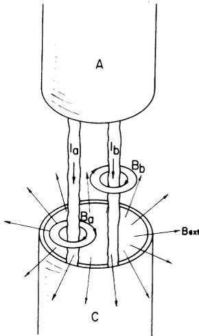
Fig. 6. Magnetic field configuration in the vicinity of two neighboring columns. Field acting on  $I_a$  is weaker than that acting on  $I_b$ .  $I_a$  moves first. A-anode, C-cathode,  $B_{ext}$  (external magnetic field),  $B_a$  (field generated by current  $I_a$ ),  $B_b$  (field generated by current  $I_b$ ).
