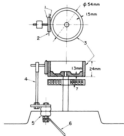
Fig. 1. Construction of trigger assembly, cathode, and spiral coil: 1) Cu sheets, 2) microscope slide cover slip, 3) cup cathode, 4) attaching screw, 5) feedthrough, 6) electrical connection, and 7) spiral coil, connected electrically in series with cup electrode. Anode assembly similarly constructed but consisting of parts 3) and 7) only.
