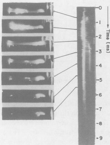
Fig. 5. Streak and frame photography of the arc without external magnetic field. Peak current is 9.3 kA at 2.9 ms. Initial capacitor voltage 200 V.
