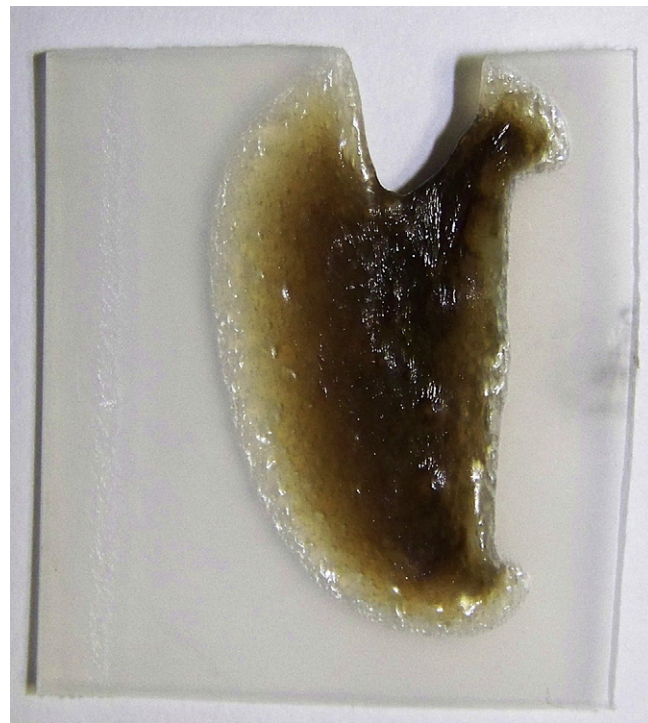
Fig. 7. Enlarged photo of the Ertalon-6 sample ( 2.0 \times 1.75 \text{ cm}^2 ) following the experiment. Note that the charred material and the visible bubbles are within the sample. The external surface of the sample is clear and smooth.
