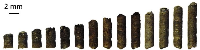
Fig. 5. An AM of a 2\text{-mm}^{\emptyset} metal rod constructed in 14 consequent steps (repeating the process shown in Fig. 4). The additive stepwise process resulted in a \sim 10\text{-mm} long rod made of solidified increments of bronze-based powder.
