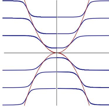
Fig. 3. Dispersion dependence  $\Omega(K)$  for a bending beam on the dynamic elastic foundation, (15). The brown curves,  $\Omega = \pm K^2$ , correspond to the free beam ( $b_0 = 0$ ). The horizontal asymptotes of the blue lines,  $K \rightarrow \pm\infty$ , reflect the resonant oscillations.
