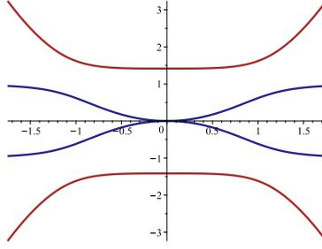
Fig. 2. Dispersion dependencies  $\omega(k)$  for a bending beam with distributed oscillators. The equation is  $(k^4 - \omega^2)(1 - \omega^2) = \omega^2$ . The upper branch can be called as for the beam under the oscillators influence, and vice versa for the lower one.
