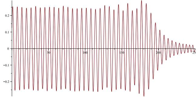
Fig. 4. The wave in a bending beam. Asymptotic representation following from the general expressions (27), (28) with nondimensional parameters  $\omega_0 = k_*$ ,  $\eta_2 = 1$ ,  $v_g = 2$ ,  $t = 100$ .
