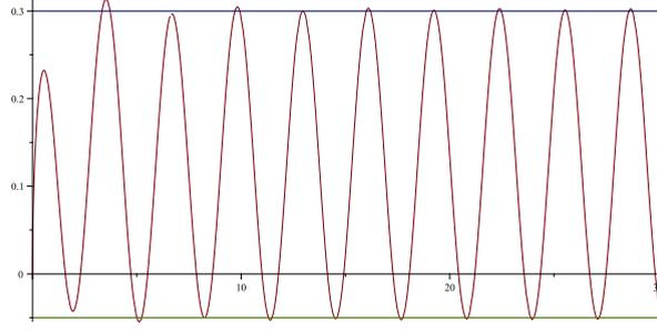
Fig. 6. The rate of the energy flux from the concentrated force to the beam.
