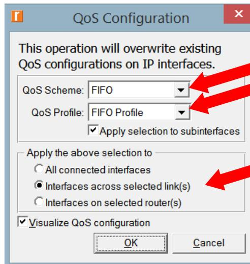
*Note:* Since the **Visualize QoS Configuration** radio button is checked, the link is colored based on the QoS scheme used.
