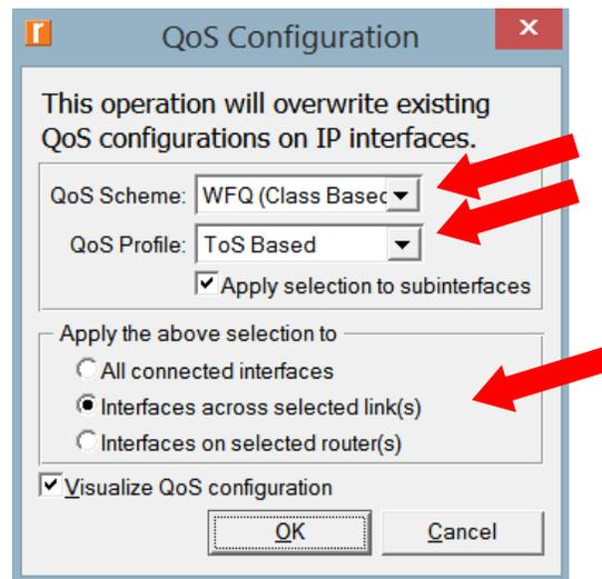
*Note:* Since the **Visualize QoS Configuration** radio button is checked, the link is colored based on the QoS scheme used.
