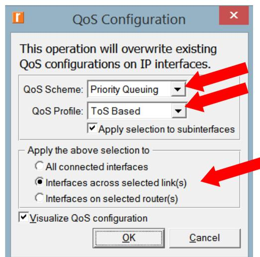
*Note:* Since the **Visualize QoS Configuration** radio button is checked, the link is colored based on the QoS scheme used.
