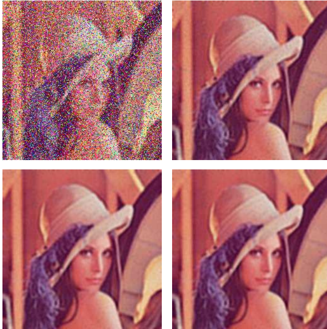
Fig. 2. Color image restoration using several regularization methods. Top-left: Blurred image with 30% impulse noise. Top-right: Beltrami flow regularization. Bottom-left: Color Mumford-Shah (MS). Bottom-right: Color TV Mumford-Shah (MSTV).
