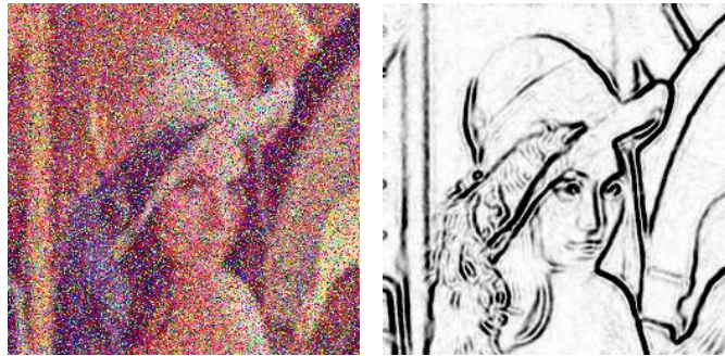
Fig. 6. Left: Blurred image contaminated by 30% impulsive noise. Right: Edge map obtained as a by-product of restoration using MS regularization.
