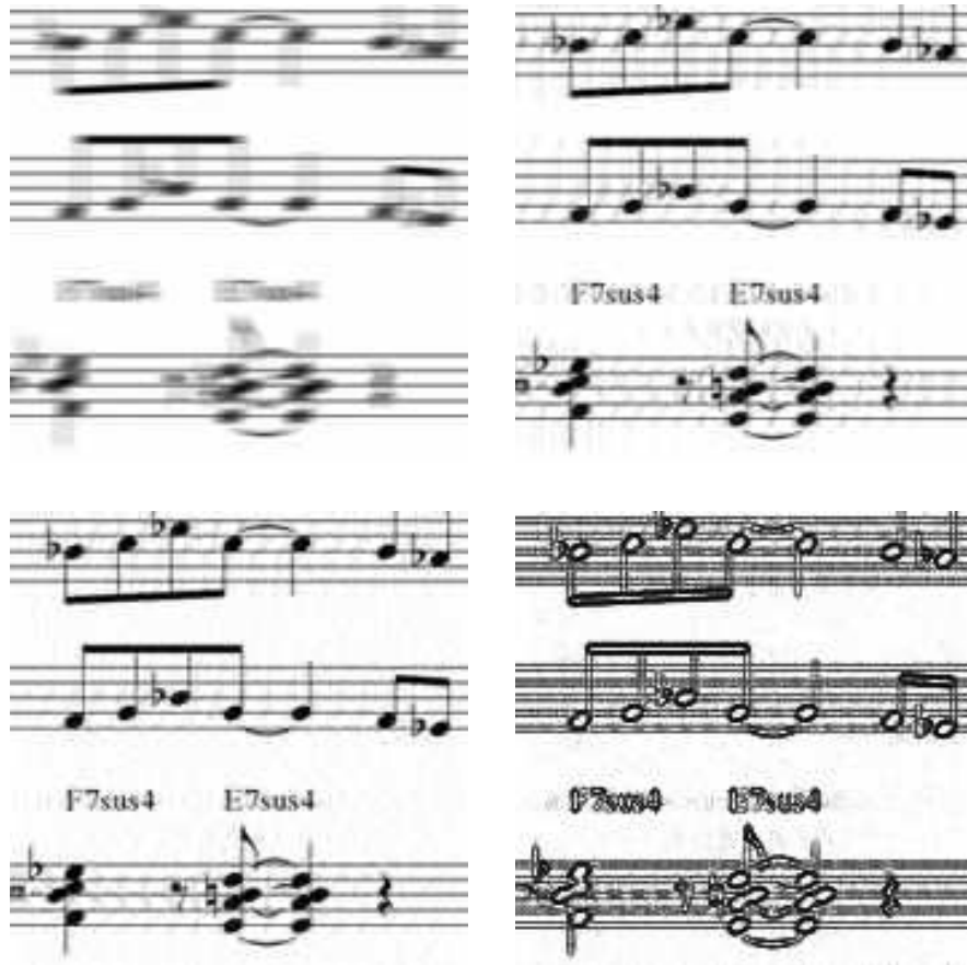
Figure 4: The case of a known (9-pixel horizontal motion) blur kernel. Top-left : Corrupted image. Top-right : Restoration using the TV method [17,24]. Bottom-left : Restoration using the suggested method. Bottom-right : Edge map produced by the suggested method.
