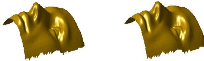
Figure 1: Left : A mannequin head shape, acquired using a Cyberware laser-based range scanner, used in this study as “ground truth”. Right : Reconstruction by (carefully tuned) photometric stereo.
