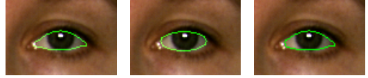
Figure 6. Left: Parabolas fitted to the upper and lower boundaries of the eye element. Middle: Ellipse fitted to the edges of eye element. Right: Segmented eye, obtained by combined use of the fitted parabolas and ellipse.
