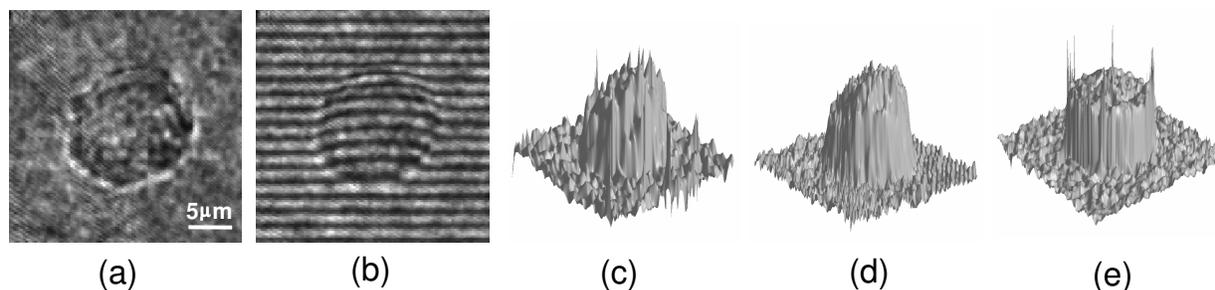
**FIGURE 2.** WFDI quantitative phase microscopy of live human skin cancer (A431, epidermoid carcinoma) cell in growth media: (a) Intensity image through the system (low visibility); (b) Single off-axis interferogram; Surface plots of the final unwrapped phase obtained by: (c) traditional off-axis geometry (old method), (d) slightly-off-axis geometry (proposed method), and (e) traditional on-axis geometry (old method) [3].
