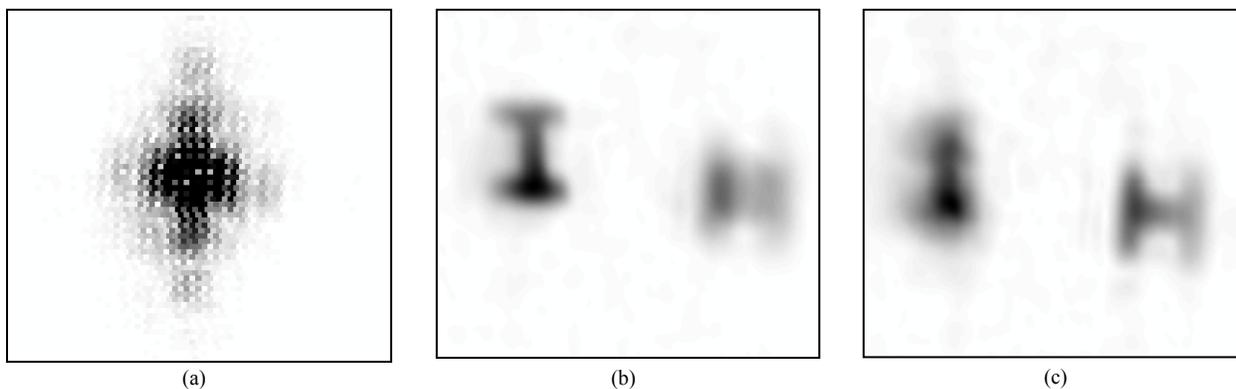
Fig. 4: (Contrast-inverted pictures) (a) Magnitude of the Fourier hologram, obtained by the processing stage. (b) Reconstruction of the hologram at the best focus distance of the letter 'I'. (c) Reconstruction of the hologram at the best focus distance of the letter 'H'.
