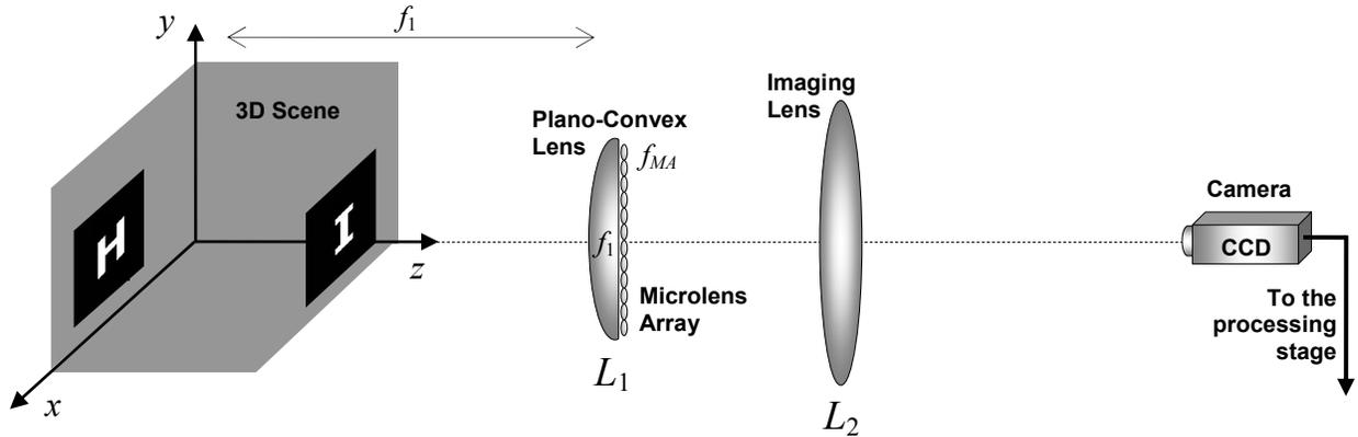
Fig. 1: The IH optical system for recording the hologram.
