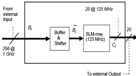
Fig. 5. A  $1 \times 256$  SLM electrical driver.
