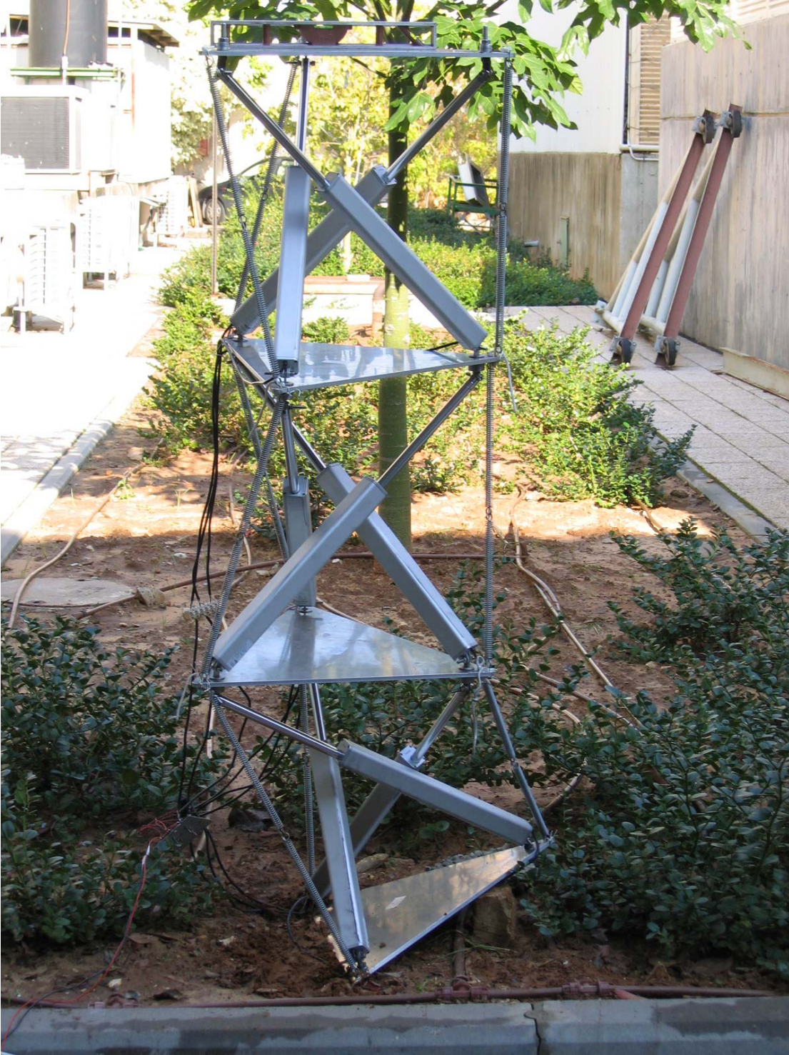
Figure 3.5: Three-staged Class 2 mast prototype.
