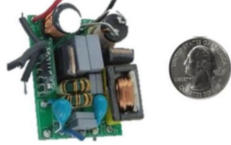
Fig. 6. View of one of the experimental prototypes. LWH =  $45 \times 30 \times 30$  [mm].
