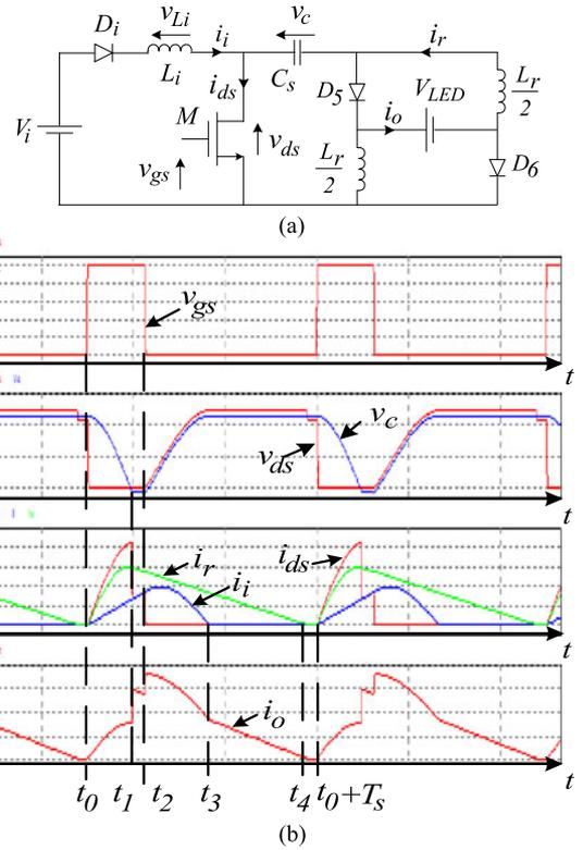
Fig. 2. (a) Equivalent circuit and (b) simulated waveforms of the proposed QRLEDD with coupled current doubler rectifier on the switching cycle scale.
