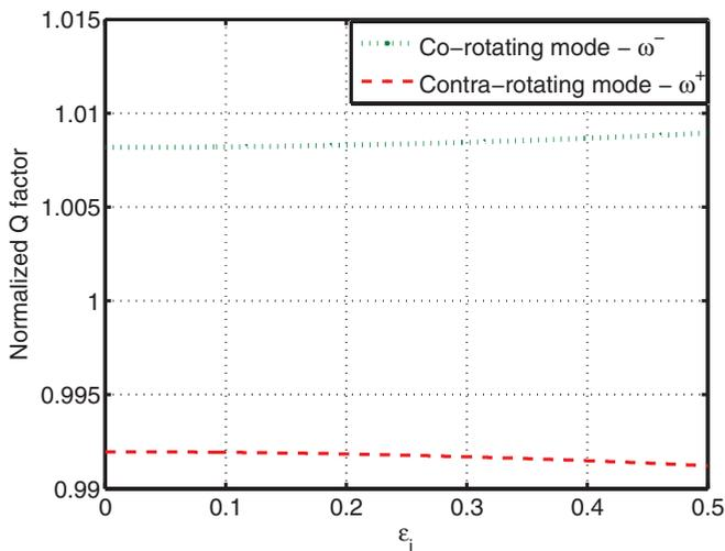
FIG. 3. (Color online) Quality factors of a rotating ring resonator normalized to the quality factor of a stationary resonator.
