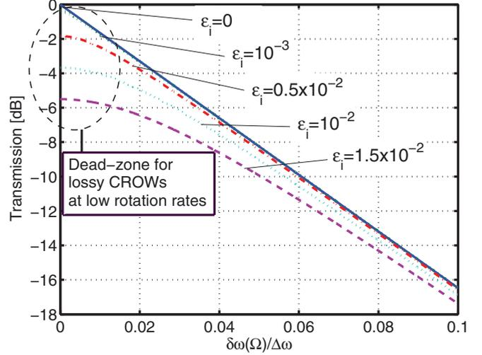
FIG. 7. (Color online) Transmission of a 20-resonator CROW for different loss values as a function of a normalized Sagnac frequency shift.
