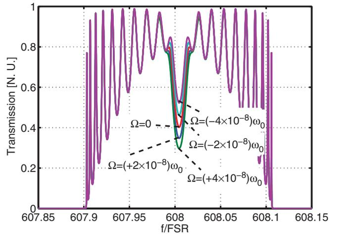
FIG. 8. (Color online) Transmission (normalized units) of a “biased” CROW as a function of frequency (normalized to the free spectral range of a single resonator with  $\omega_0$ ) for various rotation rates.
