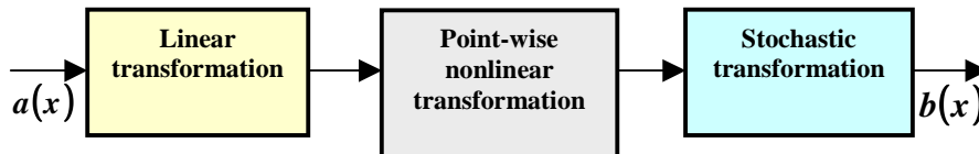
Fig. 10.1 A canonical model of imaging systems
