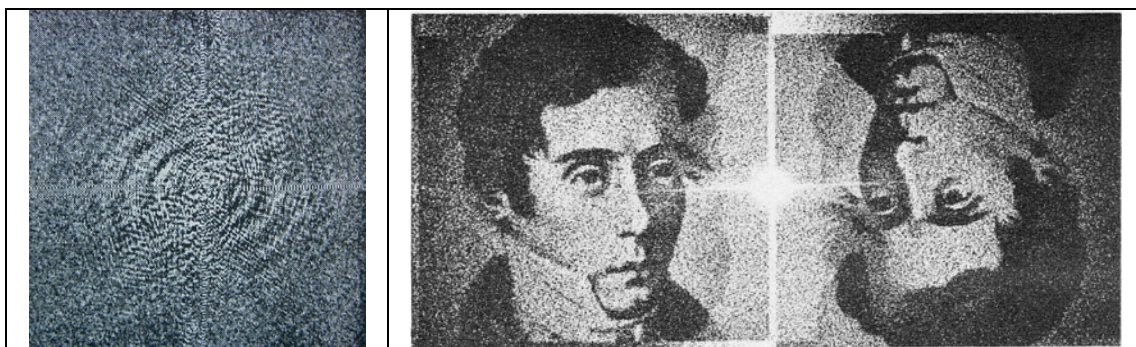
Figure 4.2. One of the first gray scale computer-generated hologram (left) and an image reconstructed from a gray scale computer-generated hologram (right, adopted from [4])
