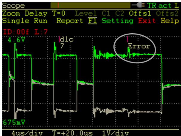
Fig. 5. A collision between the above two messages, as seen by a third passive observer. Notice that the collision begins only with the first different data bit (on  $d_0$ ), and that the dominant bits prevail. Notice also that the 12 dominant bits include the *active-error* echoed flag, identified by the observer as a *stuff-error* at the encircled red line.
