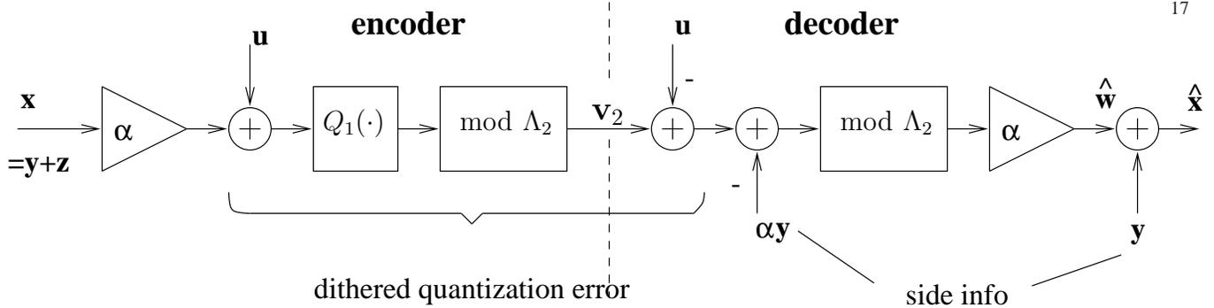
Fig. 5: Wyner-Ziv encoding of a jointly Gaussian source using nested lattice codes. At high resolution  $\alpha = 1$ .
