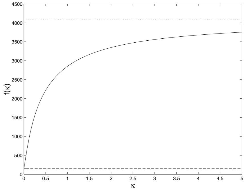
Figure 2:  $f(\kappa)$  in the case of  $\alpha = 1$  . Solid:  $f(\kappa)$ , dotted: the limit of  $f(\kappa)$  as  $\kappa \rightarrow \infty$  according to Property 4, dashed: the limit of  $f(\kappa)$  as  $\kappa \rightarrow 0$  according to Property 3. Note that the slope of  $f(\kappa)$  approaches zero as  $\kappa \rightarrow \infty$  according to Property 6. (Parameters:  $P = 0.15$ ,  $N_1 = 0.01$ ,  $N_2 = 0.1$ ,  $\rho = 3$ )
