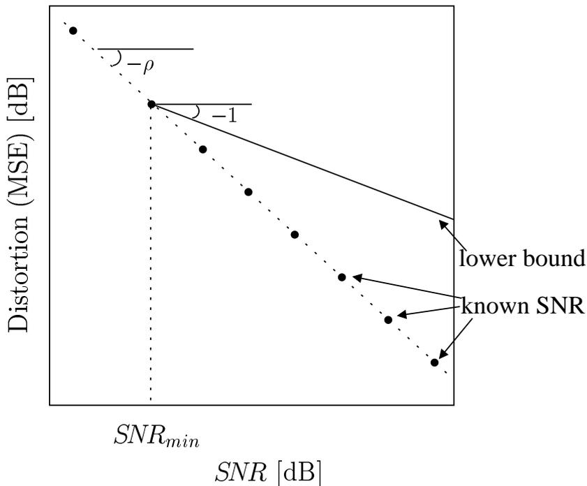
Figure 6: MSE vs. SNR. Solid: the lower bound of Corollary 3. Dotted: the solution of  $R(D) = \rho C(SNR)$
