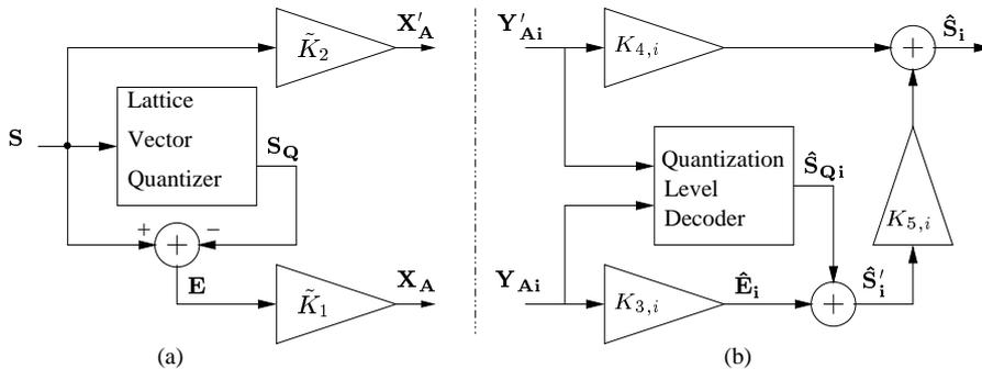
Figure 9: Modulo-Lattice modulation for lossy transmission with bandwidth expansion. (a) Transmitter. (b) Receivers ( $i = 1, 2$ )
