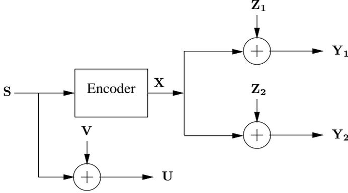
Figure 5: The Gaussian broadcast channel with the auxiliary variable  $\mathbf{U}$ .
