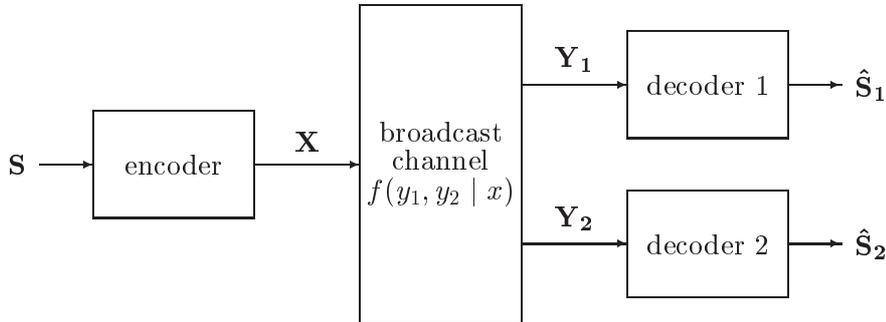
Figure 1: Lossy transmission of a source through a broadcast channel
