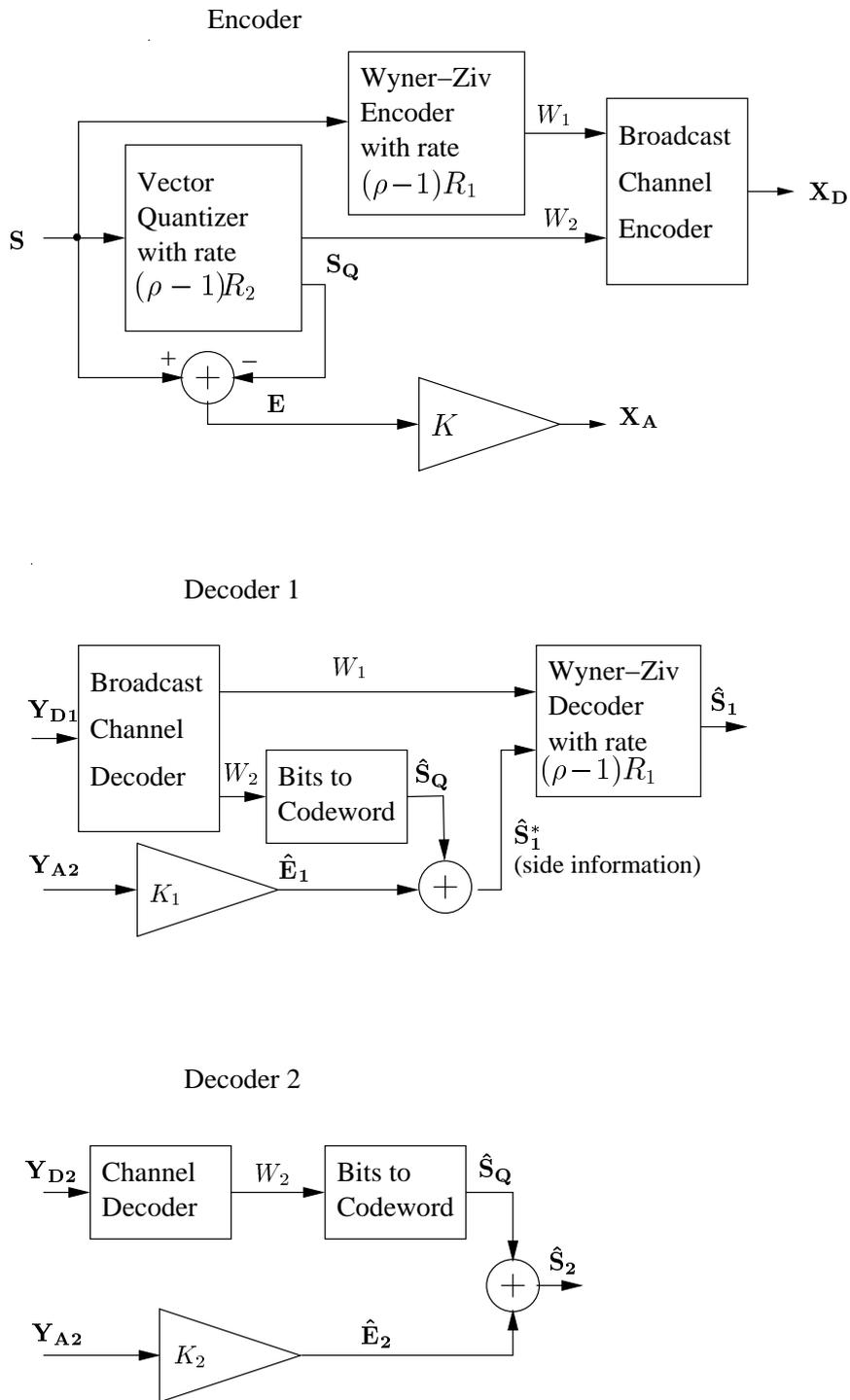
Figure 7: A coding scheme for lossy transmission with bandwidth expansion
