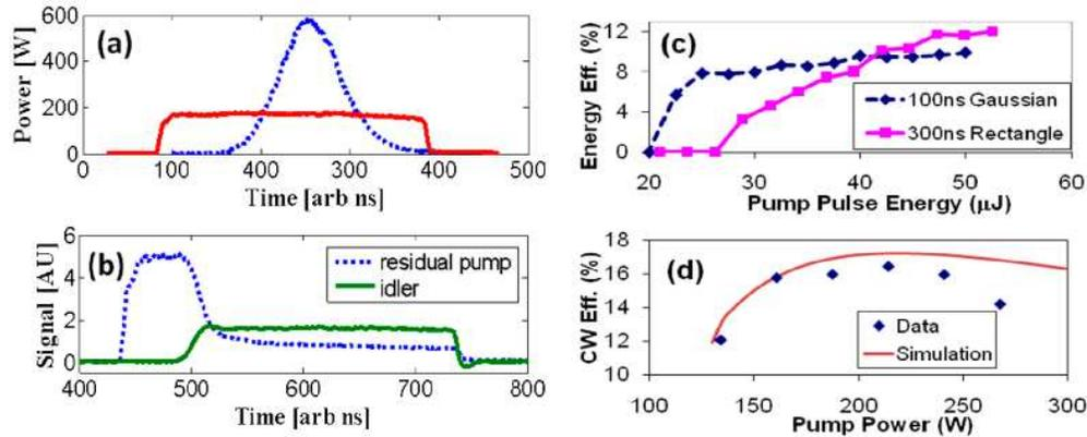
Fig. 4. OPO experimental results (a) Input pumps: Gaussian and rectangular. (b) Input and output OPO pulses in the case of rectangular pump pulse (c) OPO idler power curve for Gaussian and rectangular pulses. (d) Steady state idler conversion efficiency for rectangular pulse.
