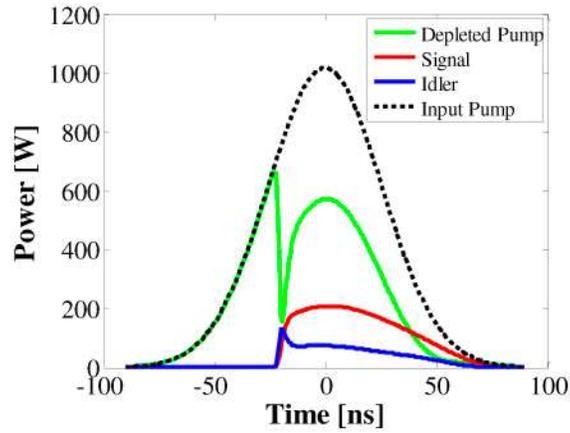
Fig. 1. OPO performance with a 60ns Gaussian pulse.
