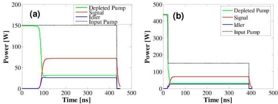
Fig. 3. Temporal evolution of pump, signal, and idlers pulses: (a) rectangular pulse, (b) optimized double rectangular pulse.
