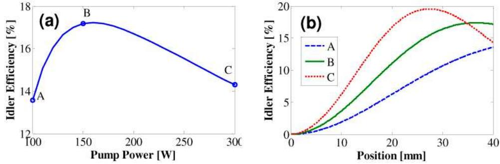
Fig. 2. OPO performance with a rectangular pulse. (a) Idler steady-state efficiency. (b) Steady-state idler efficiency within the crystal for pump power of (A) 100W, (B) 150W and (C) 300W.
