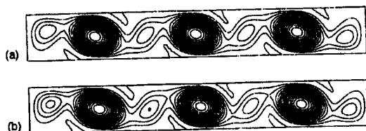
FIGURE 4 Three-roll steady state flows. A = 7.25 , Pr = 0 . Calculation using the Galerkin method, 60 \times 20 basis functions. (a) Gr = 4.9 \times 10^5 (point S_3 in Fig. 1c), (b) Gr = 5.2 \times 10^5 (point N_4 in Fig. 1c).
