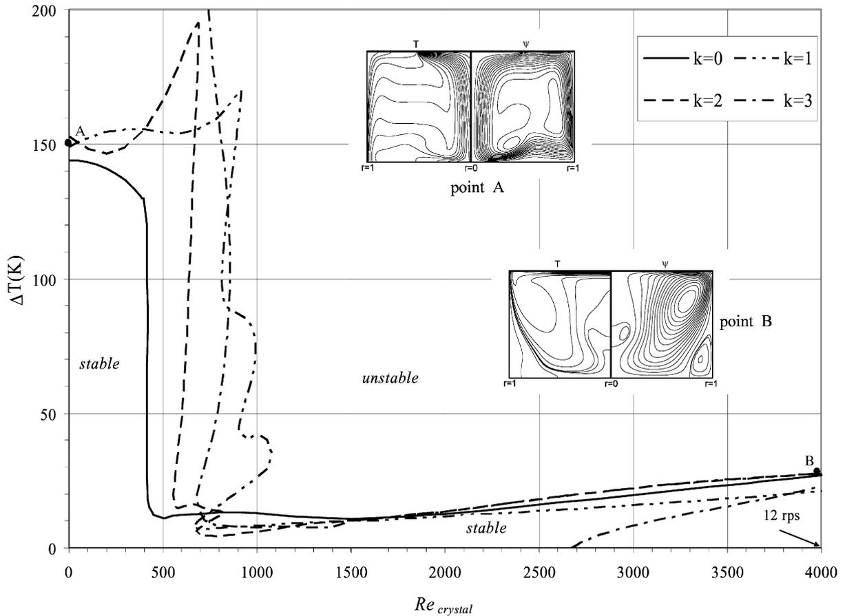
Fig. 2. Stability diagram of the melt flow in the Czochralski configuration considered in Ref. [1].
