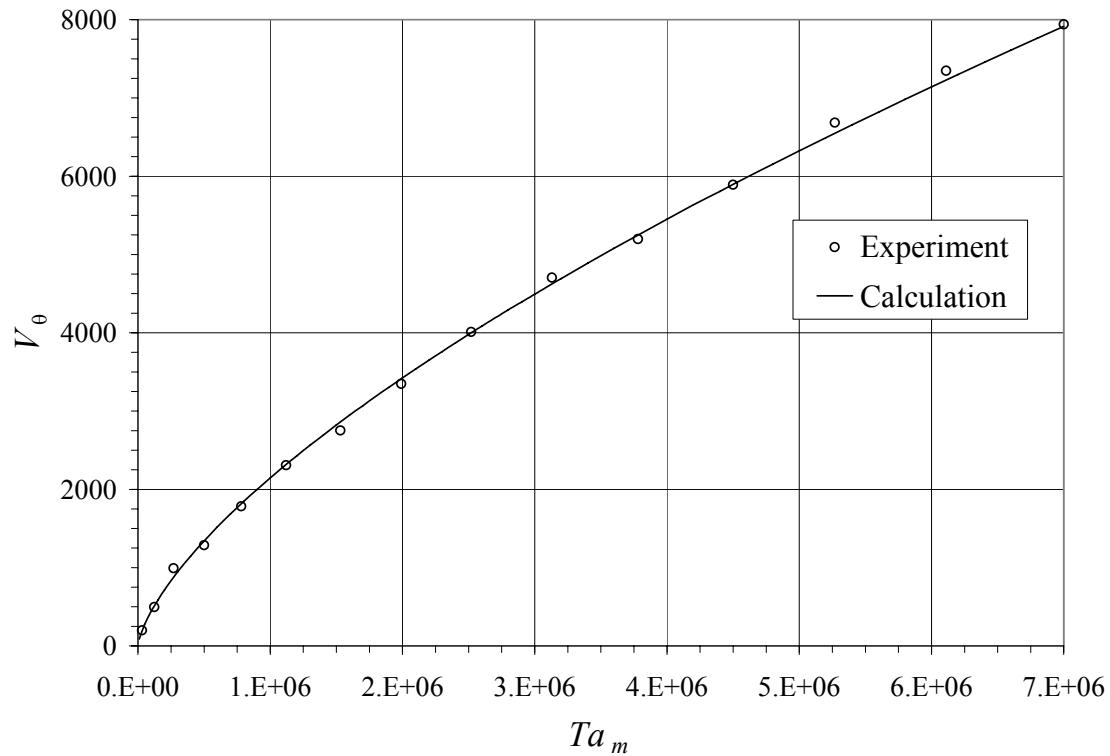
Fig.6. Dependence of the dimensionless azimuthal velocity on the RMF Taylor number in the point  $r = R/2$ ,  $z = H/2$ . Calculation and measurements for  $H/R = 2$ ,  $B = 2.1$  mT,  $Ta_m = 3.03 \times 10^6$ ,  $Ha = 2.58$ .
