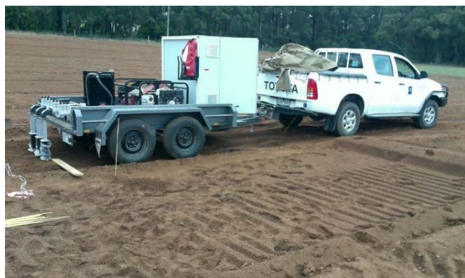
Figure 4: A 4x2 kW microwave trailer prototype in the field.
