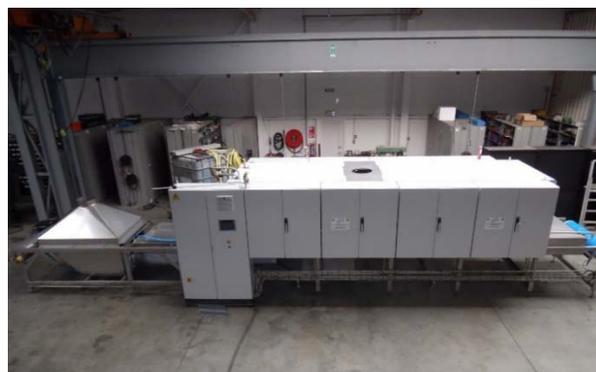
**Figure 2.** The MEAM Dry S48 HR (the S stands for Sheet and HR for Heat Recovery) with a maximum power of 48 kW.
