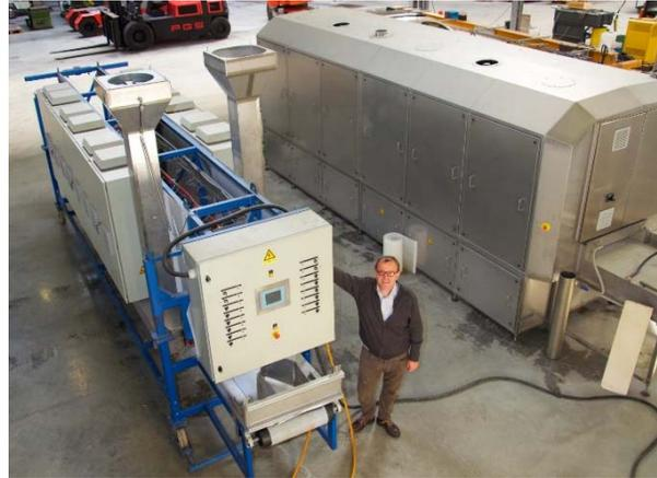
**Figure 1.** Two industrial microwave systems: the MEAM Dry 32 (left) and the MEAM Dry S20 (right). The number reflects the maximum power of the machines.
