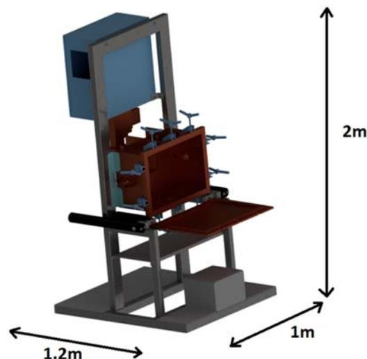
**Figure 3.** Drawing of the MEAM VP 1.2 (VP and 1.2 stand for vacuum/pressure and 1.2 kW power, respectively).
