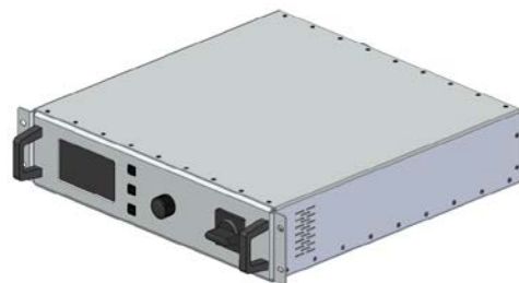
Figure 6. Concept rendering of the SSMG to be introduced by Muegge (courtesy Muegge GmbH).
