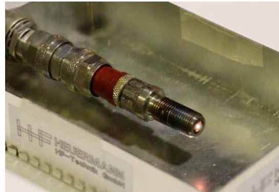
Figure 4. Prototype coaxial resonator for plasma automotive ignition 8 .
