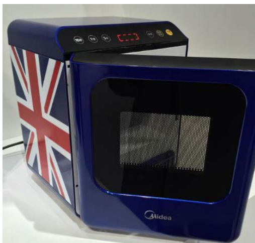
Figure 3. Microwave oven with solid state RF source developed jointly by Midea and NXP 6 .
